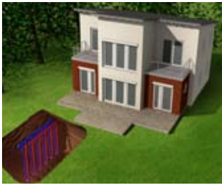
Vertical Ground Loop System
